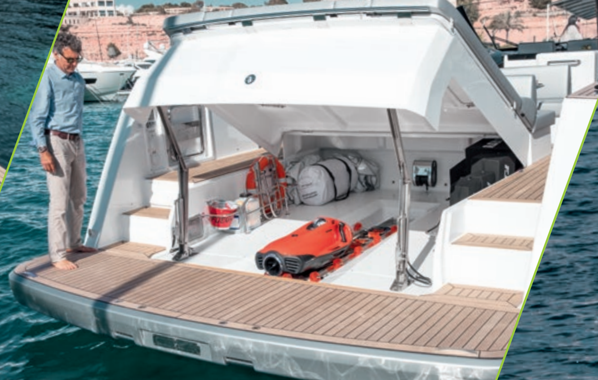
large garage for jet tender and water sports devices, hydraulically opened
