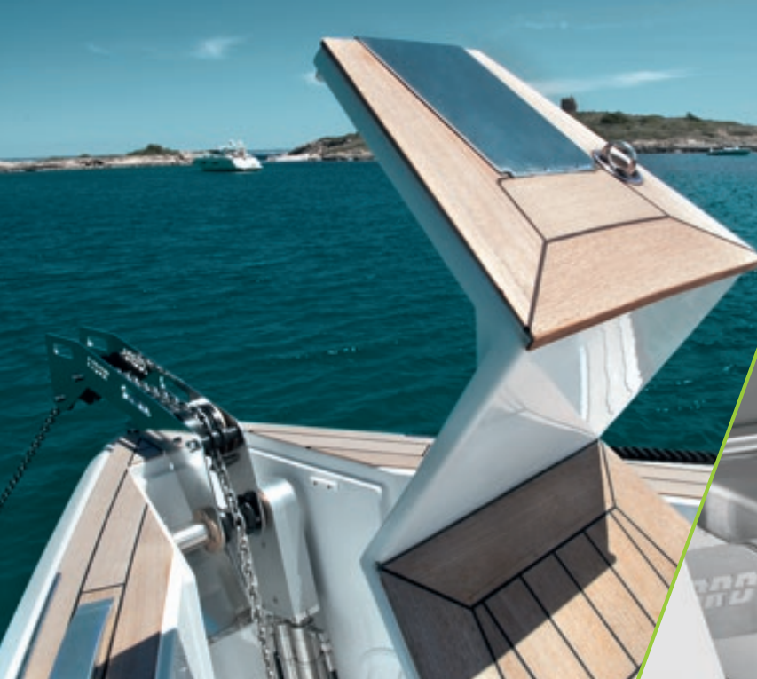
easy to use: the hydraulic anchor launching system
